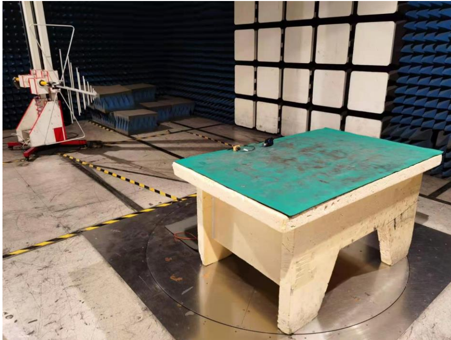
Spurious Emission Test Setup (Below 1GHz)
