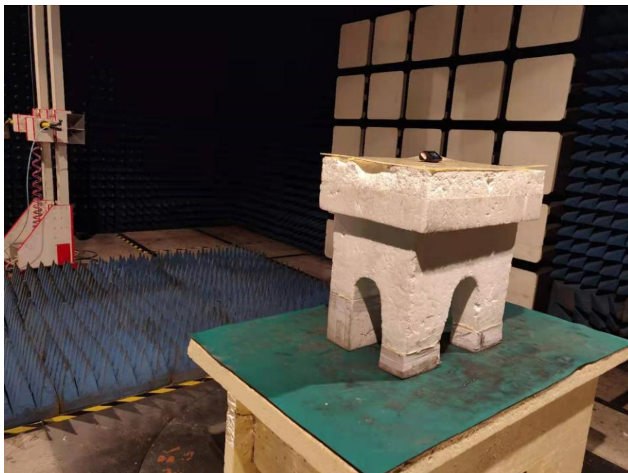
Spurious Emission Test Setup (Above 1GHz)
