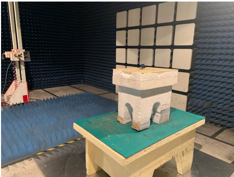
Spurious Emission Test Setup (Above 1GHz)
