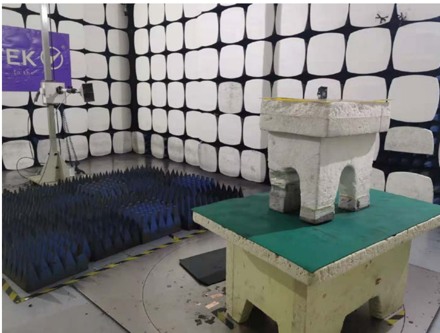
Spurious Emission Test Setup (Above 1GHz)
