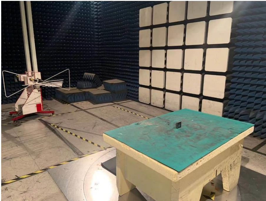
Spurious Emission Test Setup (Below 1GHz)
