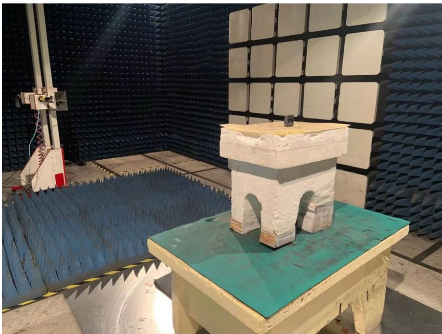
Spurious Emission Test Setup (Above 1GHz)
