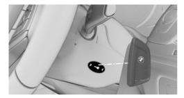
The drive-ready state cannot be switched on if the remote control has not been detected. If this happens, proceed as follows:
