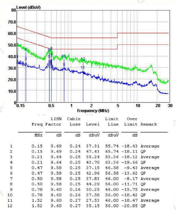
Remark: Factor = Insertion Loss + Cable Loss, Result = Reading + Factor, Margin = Result – Limit.
