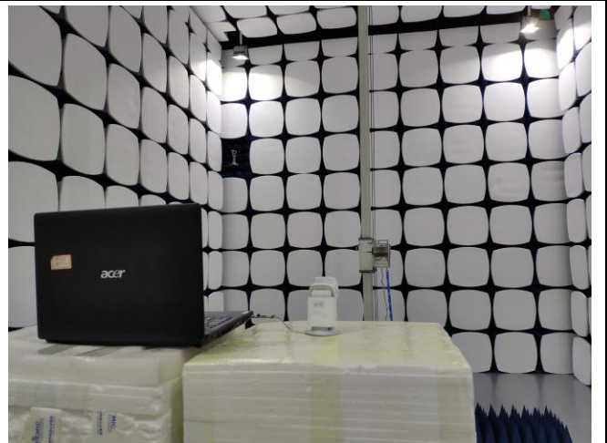
Radiated Spurious Emissions Test Setup Above 1GHz
