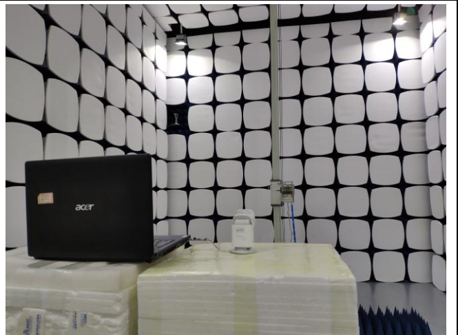
Radiated Spurious Emissions Test Setup Above 1GHz
