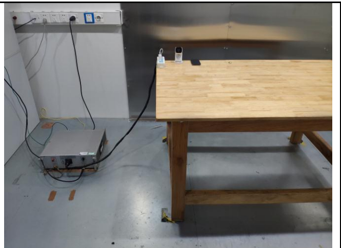
Conducted Emissions Test Setup Side View
