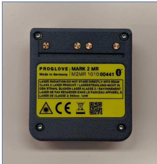
Figure 2: MARK 2 Label Position at the bottom side of the scanner
