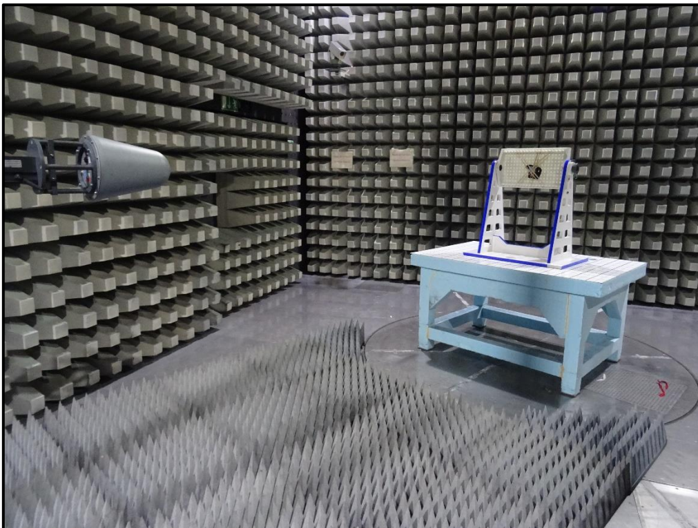
Photo 6: Radiated Test Setup-1 GHz to 18 GHz
