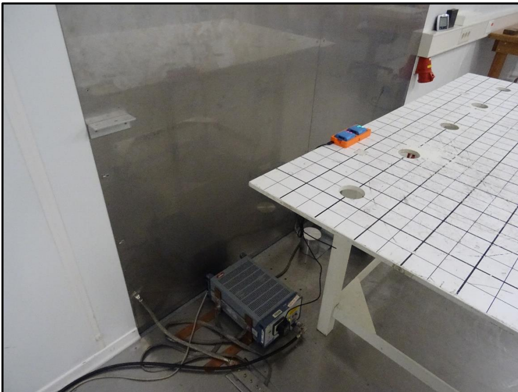
Photo 12: AC Conducted Emissions Test Setup
