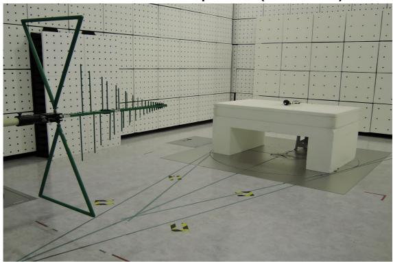
Radiated Emission Set up Photos (Above 1GHz)
