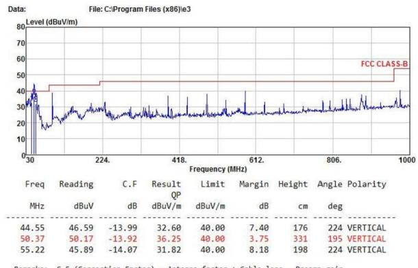
Remarks: C.F (Correction Factor) = Antenna factor + Cable loss - Preamp gain
