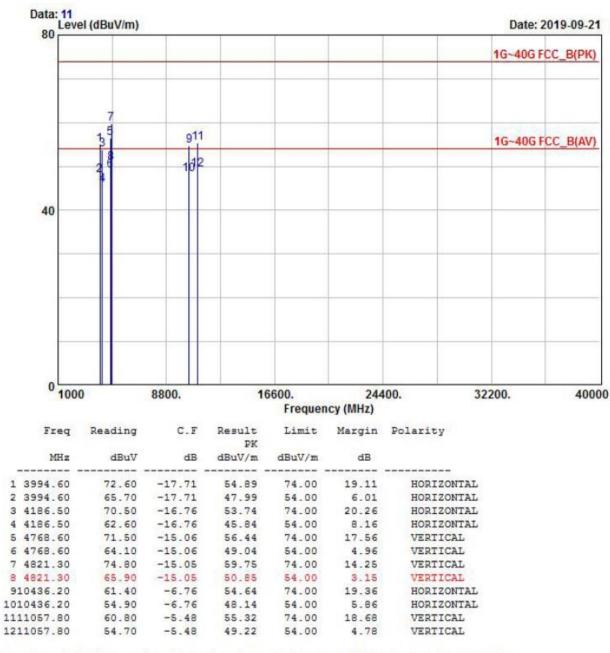
Remarks: C.F (Correction Factor) = Antenna factor + Cable loss - Preamp gain Blue : Vertical Black : Horizontal
