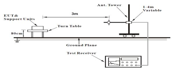
3. Radiated Emission Test Set-Up, Frequency Above 1000 MHz.
