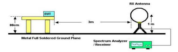
2. Radiated Emission Test Set-Up, Frequency Below 1000 MHz
