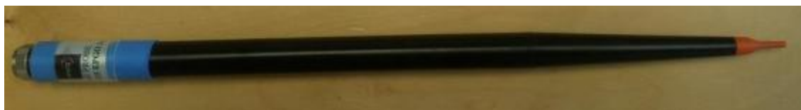
Figure-MVG COMOSAR Dosimetric E field Dipole
