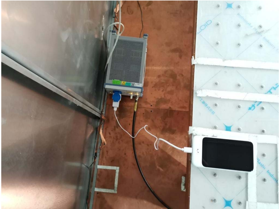
Conducted Emissions Test Setup (with charger)
