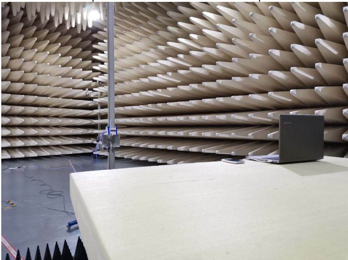
Spurious Radiated Emissions Test setup
