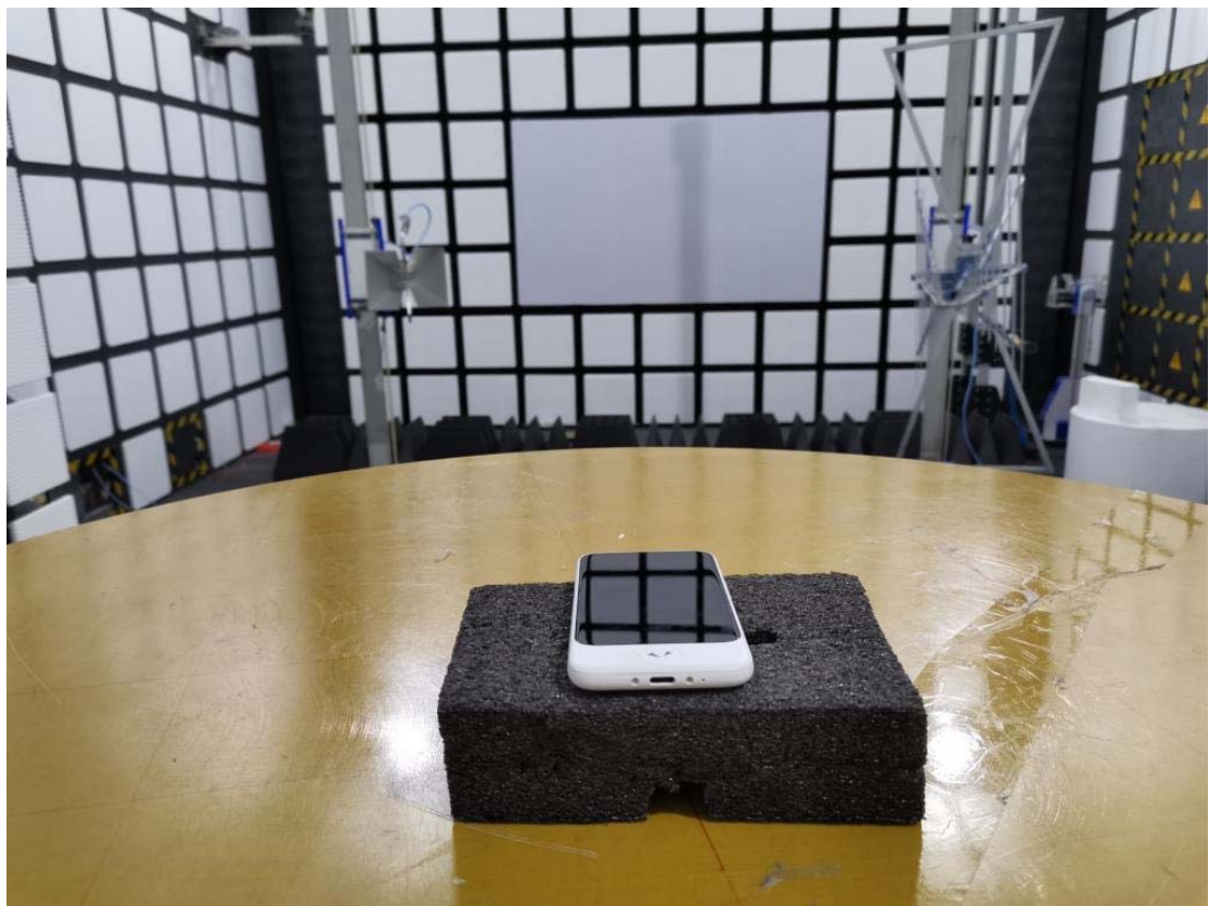
Spurious Radiated Emissions Test setup
