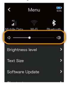
You can also adjust the volume with the volume button on the right side of the unit.
