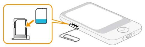
Mount a nano SIM card onto the SIM card slot, and insert it into the unit.
