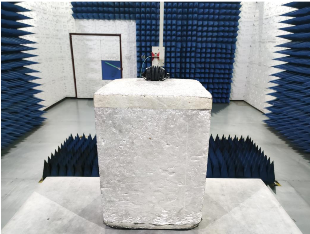
RADIATED EMISSION TEST SETUP ABOVE 1GHz
