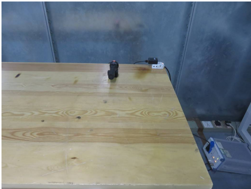
Photo of Power Line Conducted Emissions Measurement
