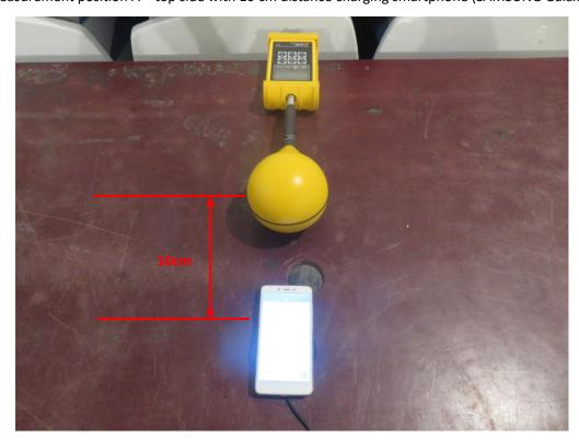
DUT – measurement position B – left side with 10 cm distance charging smartphone (SAMSUNG Galaxy S7)
