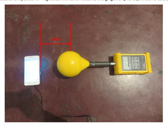
DUT – measurement position E – front side with 10 cm distance charging smartphone (SAMSUNG Galaxy S7)
