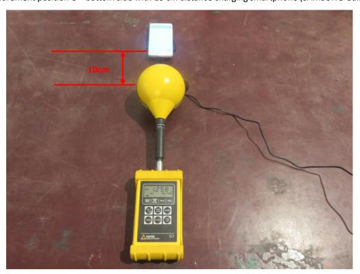
DUT – measurement position D – right side with 10 cm distance charging smartphone (SAMSUNG Galaxy S7)
