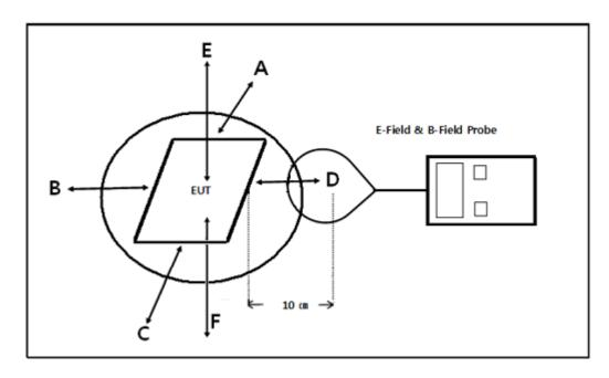
Due to installation limitations no tests from the underside of the charging device (Test Position F) are required.
