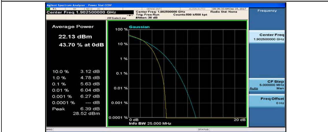
(Channel Bandwidth:15 MHz)_HCH_16QAM_75RB#0
