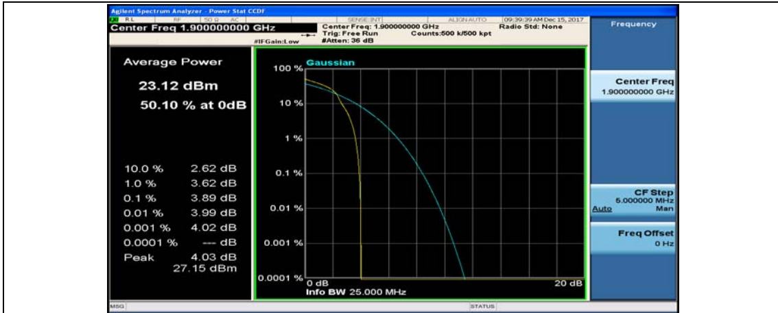
(Channel Bandwidth:20 MHz)_HCH_16QAM_1RB#99
