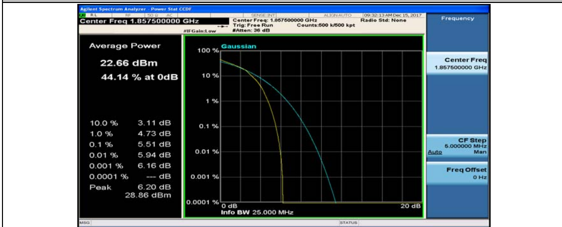
(Channel Bandwidth:15 MHz)_LCH_16QAM_37RB#38
