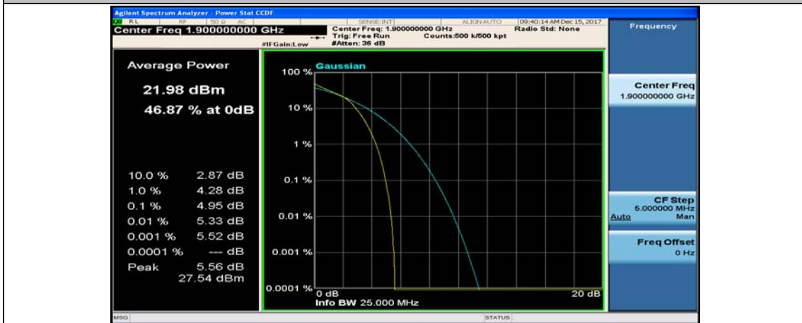
(Channel Bandwidth:20 MHz)_HCH_16QAM_50RB#25
