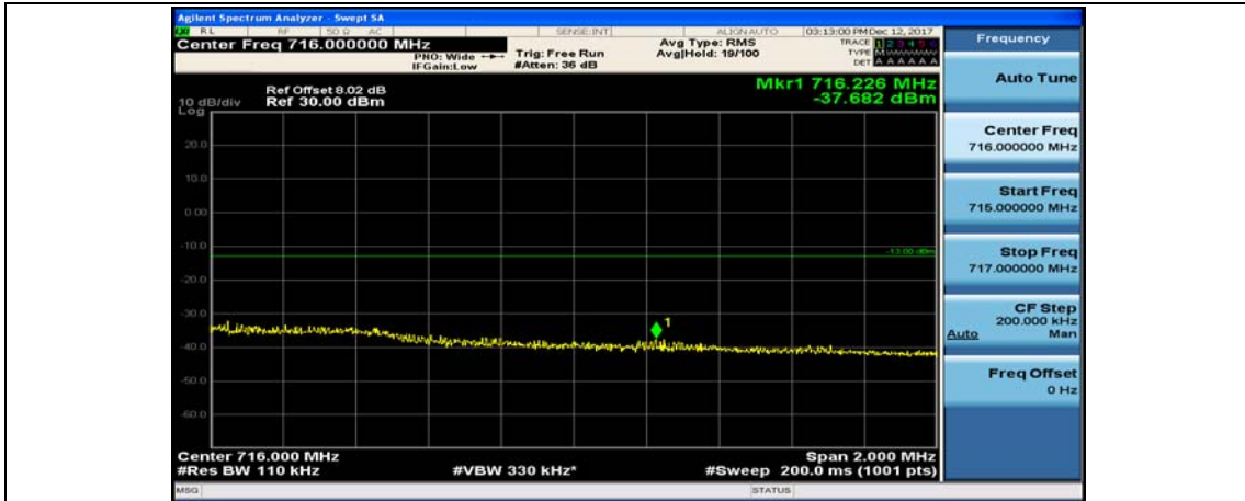
Channel Bandwidth: 10 MHz_HCH_16QAM_25RB#12
