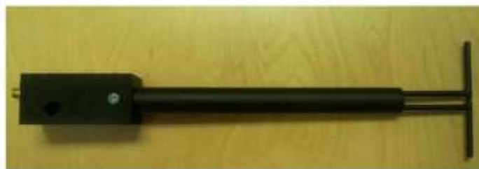
Figure 1 – MVG COMOSAR Validation Dipole
