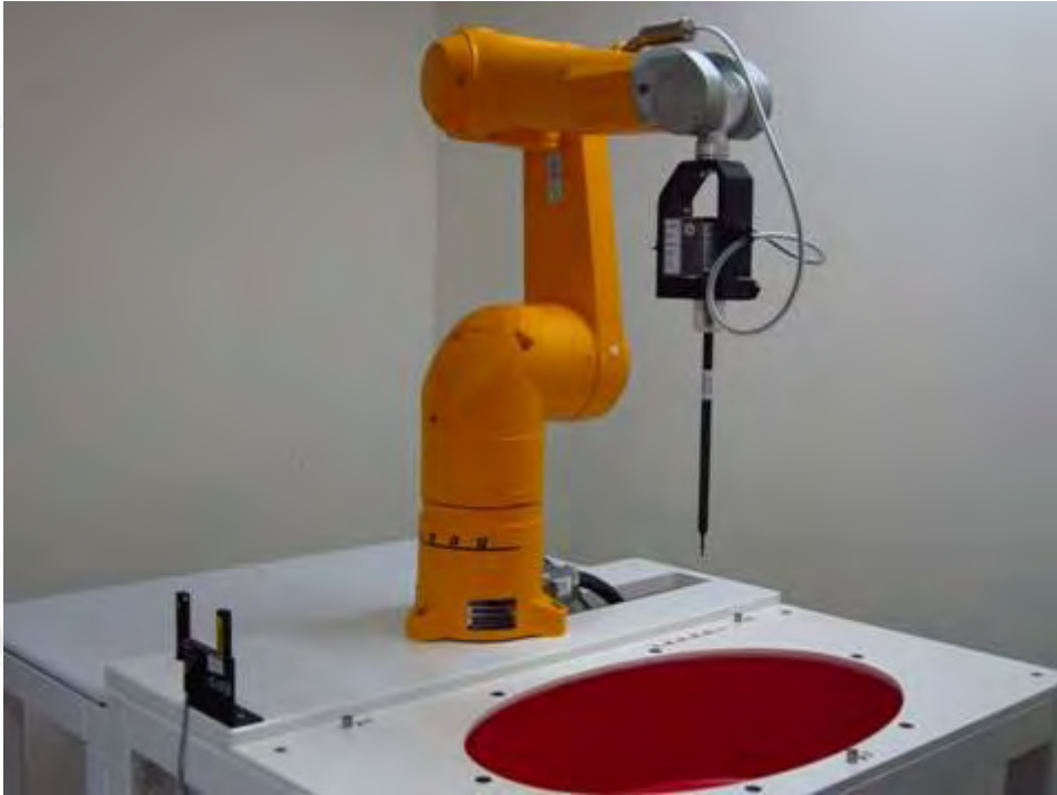
Fig.1 Photograph of the SAR measurement system
