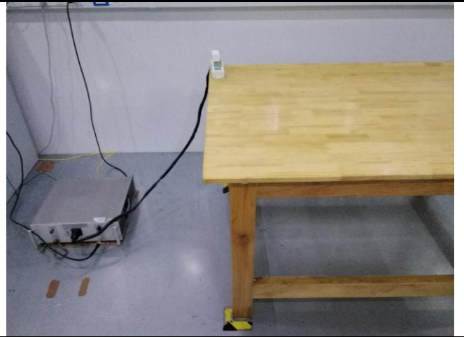
Conducted Emissions Test Setup Side View
