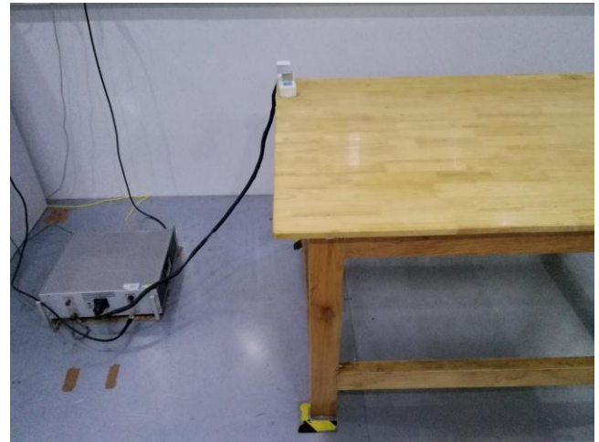
Conducted Emissions Test Setup Side View
