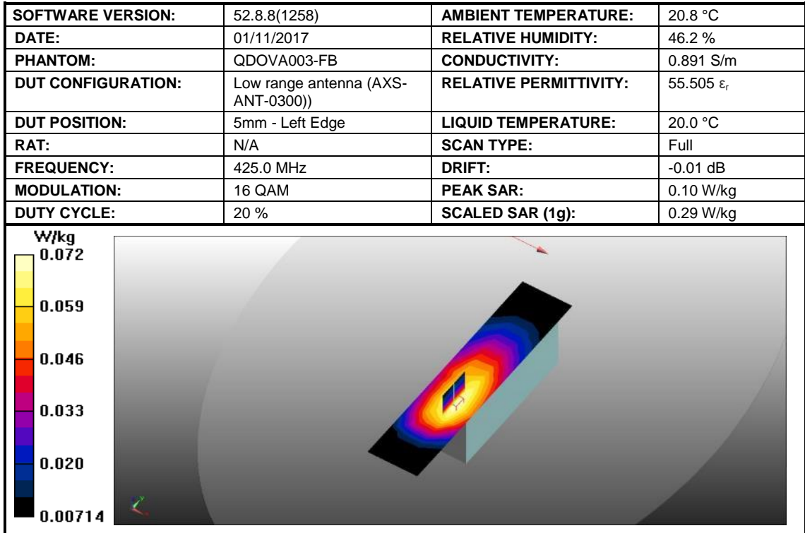
Figure 7: SAR Body Testing Results for PNG MP50 Transceiver at 425.0 MHz.
