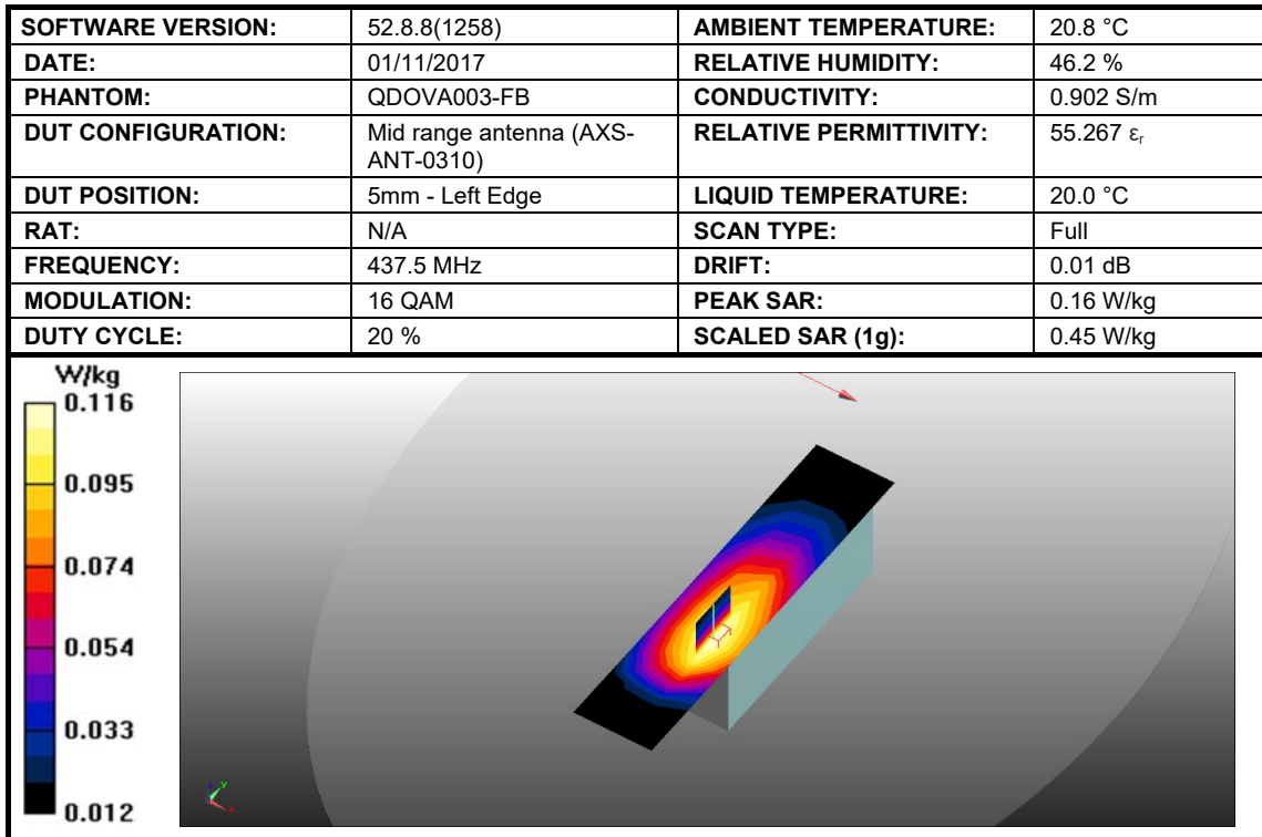
Figure 10: SAR Body Testing Results for PNG MP50 Transceiver at 437.5 MHz.
