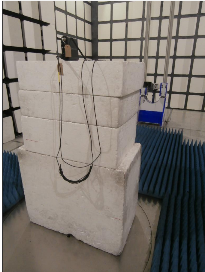
Figure 28 - Test Setup - 1 GHz to 5 GHz, Z Orientation
