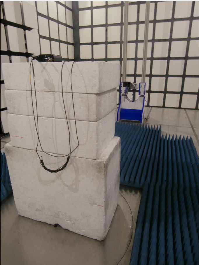
Figure 26 - Test Setup - 1 GHz to 5 GHz, X Orientation
