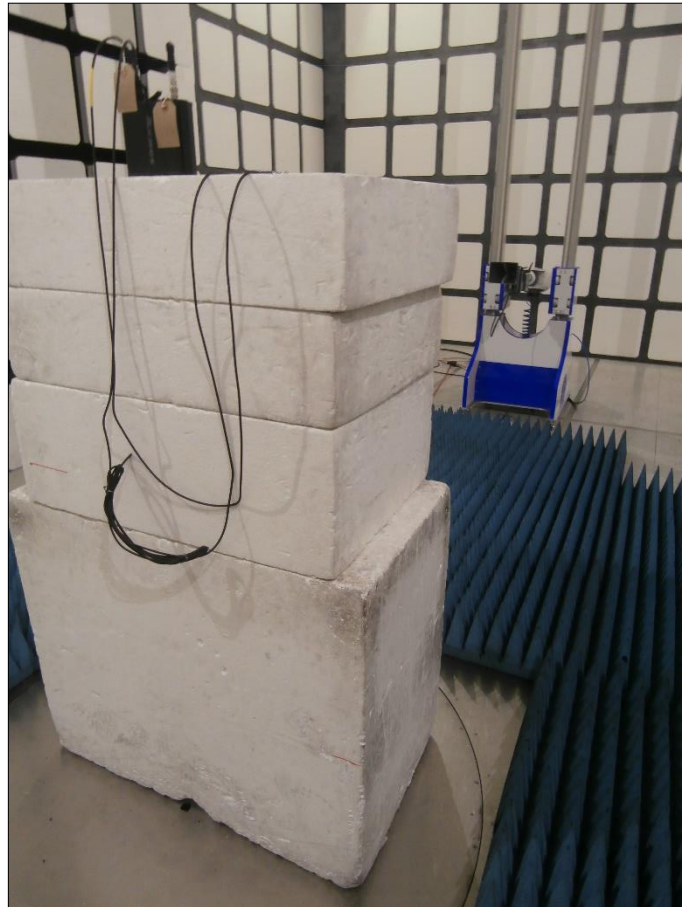
Figure 27 - Test Setup - 1 GHz to 5 GHz, Y Orientation
