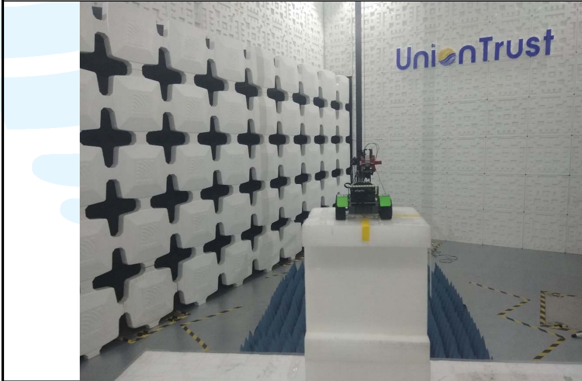
Radiated emission Test Setup (Above 1 GHz)
