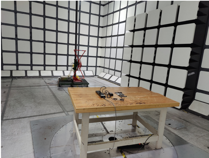
Radiated Emissions View (Below 1 GHz)
