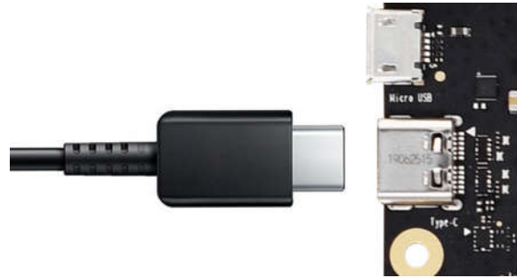
Figure 2-5. USB Type-C Port Connection
