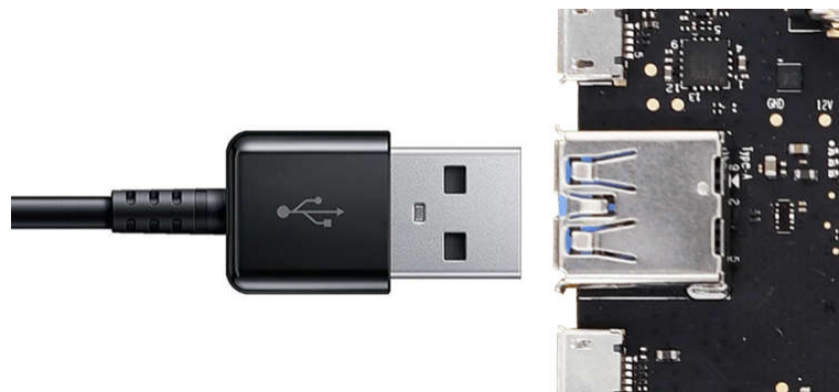
Figure 2-6. USB Type-A Port Connection
