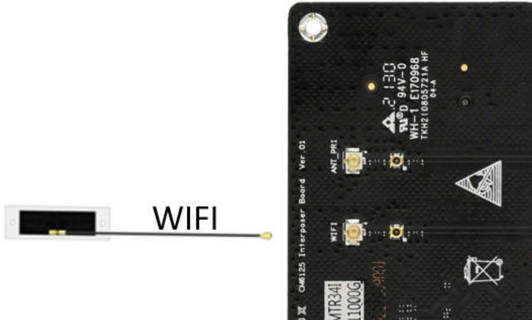
Figure 2-11. Wi-Fi/BT Antenna Connector
