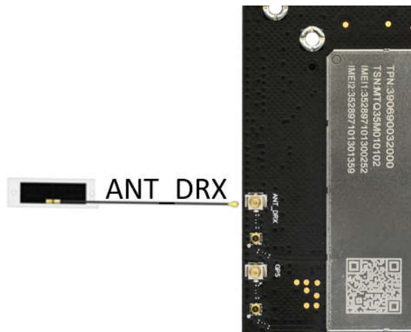
Figure 2-14. DRX Antenna Connector
