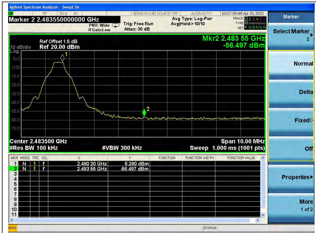
(Band edge, Channel 78, GFSK)
