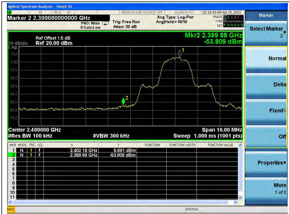
(Band edge, Channel 0, 8-DPSK)
