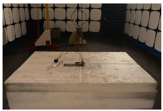
3. Radiated emission (9KHz-30MHz)
