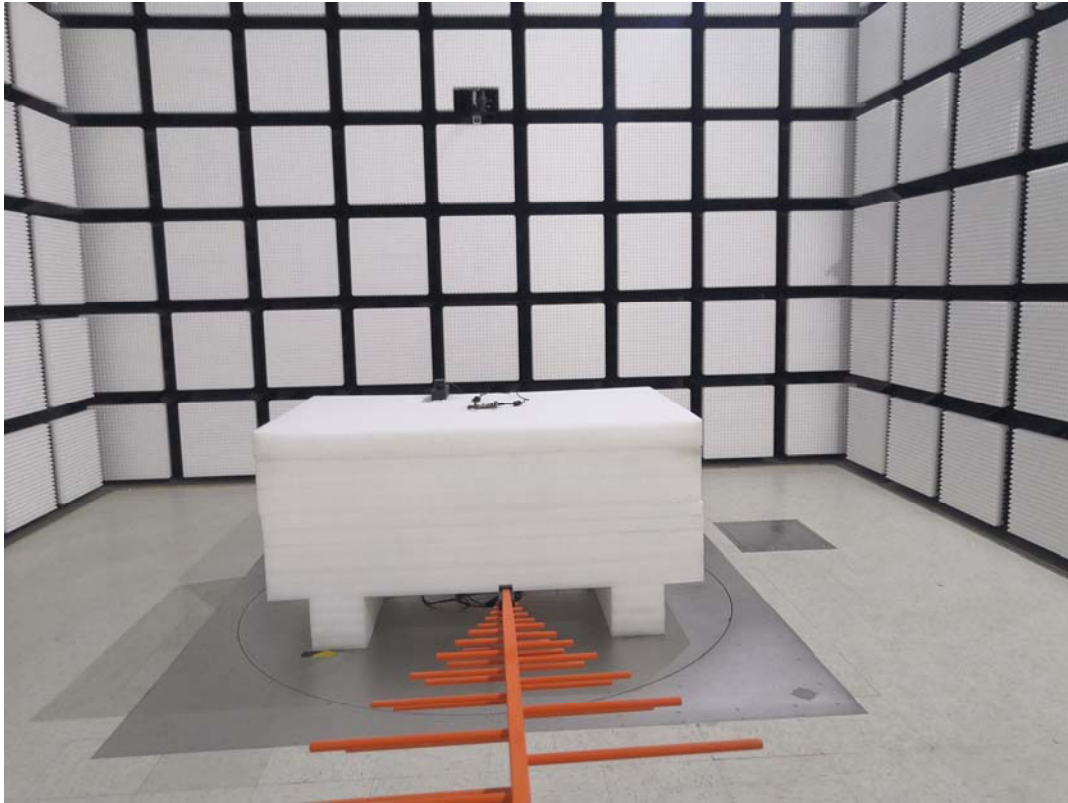
Radiated Emissions Below 1G View
