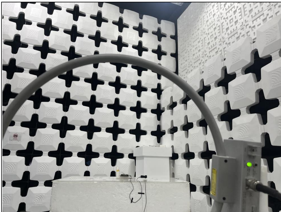
Radiated emission test: Frequency Range < 9KHz- 30MHz >
