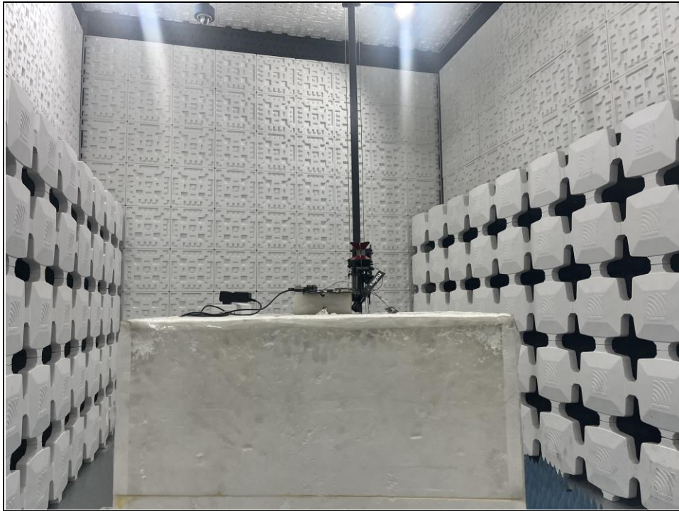
Radiated emission test: Frequency Range < 9KHz- 30MHz >
