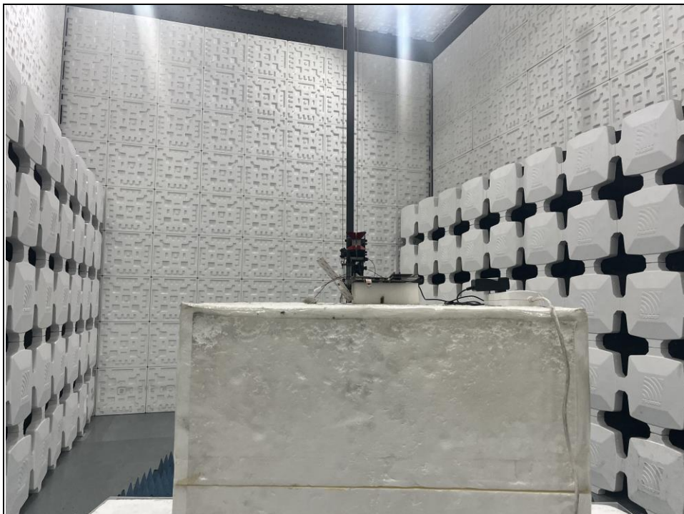
Radiated emission test: Frequency Range < Above 1GHz >
