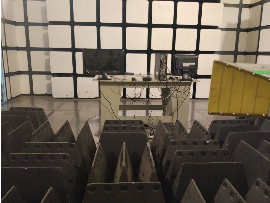
Radiated Emissions – Front View (Above 1 GHz)
