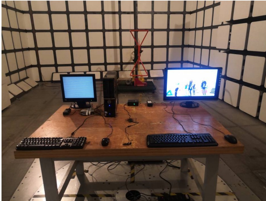
Radiated Emissions – Front View (Below 1 GHz)
