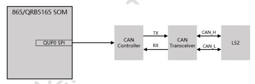
The CAN signals are rounded from CAN transceiver which is from SPI translation. The signals are:
