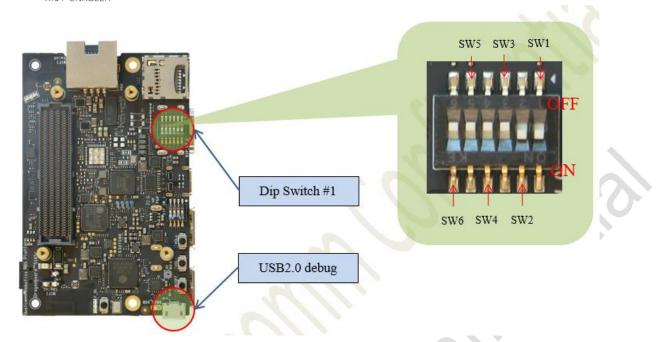
4. Connect the USB cable Micro-B plug to the USB2.0 debug port (see section 1.2.2, #21), and connect the other end to an available USB port on the host PC.
