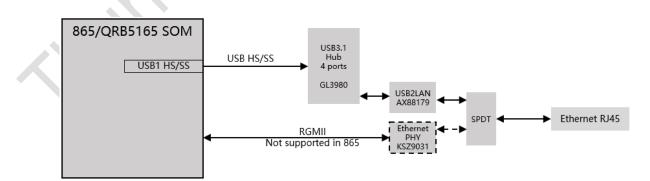
RB5 has the translation from USB1, a USB HUB and a USB to Gigabit Ethernet controller. RB5 uses an RJ45 (see Section1.2.1, #9) as the physical interface.
