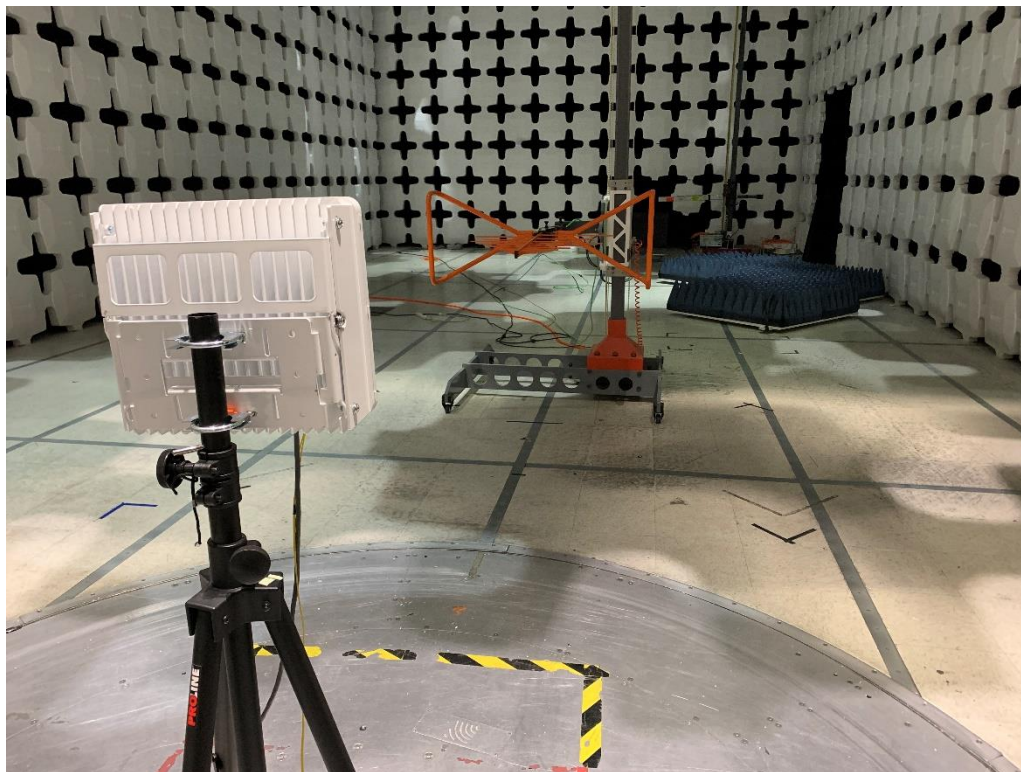
Radiated Emissions below 1GHz Front View
