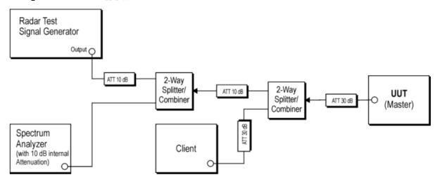
b. Set-up B is a set-up whereby the UUT is an RLAN device operating in slave mode, with or without Radar Interference Detection function. This set-up also contains an RLAN device operating in master mode. The radar test signals are injected into the master device. The UUT (slave device) is associated with the master device. Figure 5 shows an example for Set-up B. The set-up used shall be documented in the test report.
