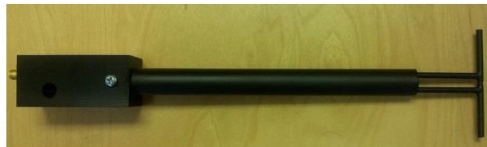
Figure 1 – MVG COMOSAR Validation Dipole
