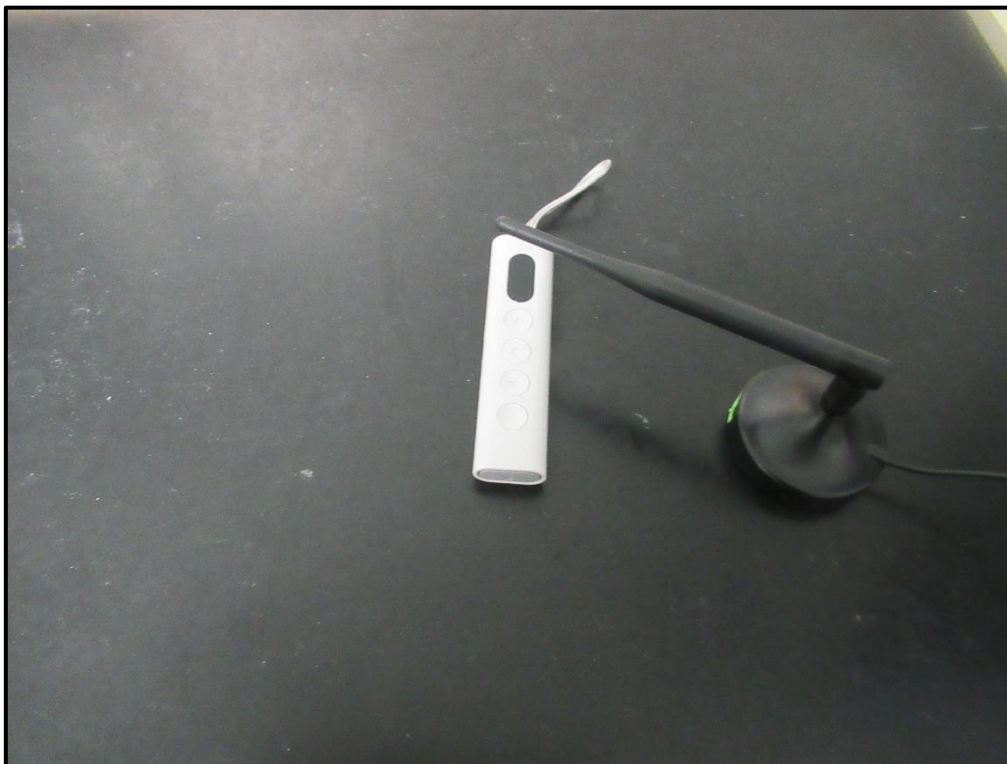
Photo 7 Test Setup for Transmitter behaviour (Periodic Operation)
