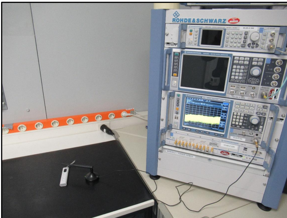
Photo 8 Test Setup for Transmitter behaviour (Periodic Operation)
