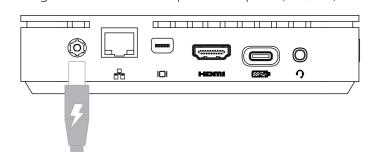
2.) By connecting to a USB-PD power source (e.g. USB-C monitor, USB-PD
