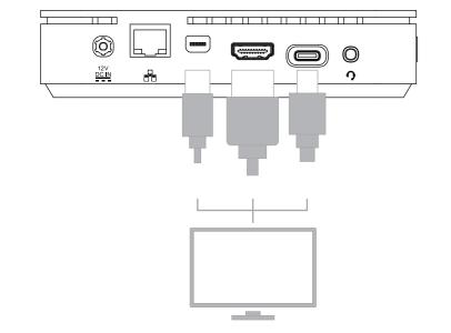
NOTE: The USB-C video output does NOT support hot-plug and does NOT contain native audio signal (this is a physical limitation of eDP signal).
