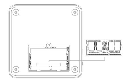
NOTE: GLK-UC2X supports 1 x 8GB DDR4 SODIMM (single-channel), or 2 x 4GB DDR4 SODIMM (dual-channel)
