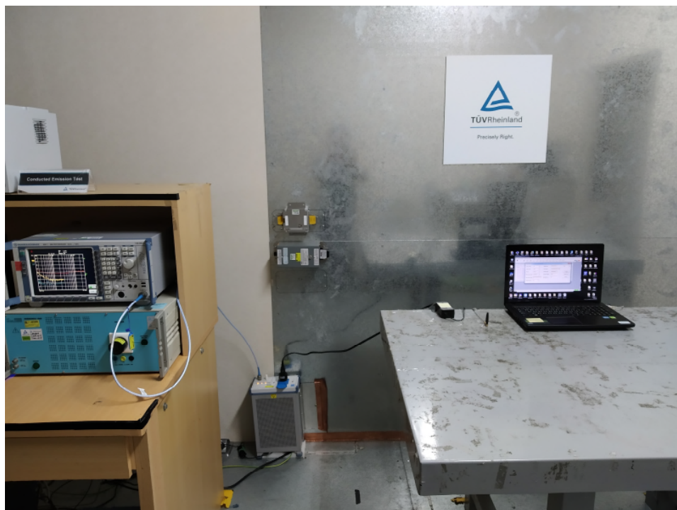
Photograph 8: Set-up for for Mains Conducted testing Front
