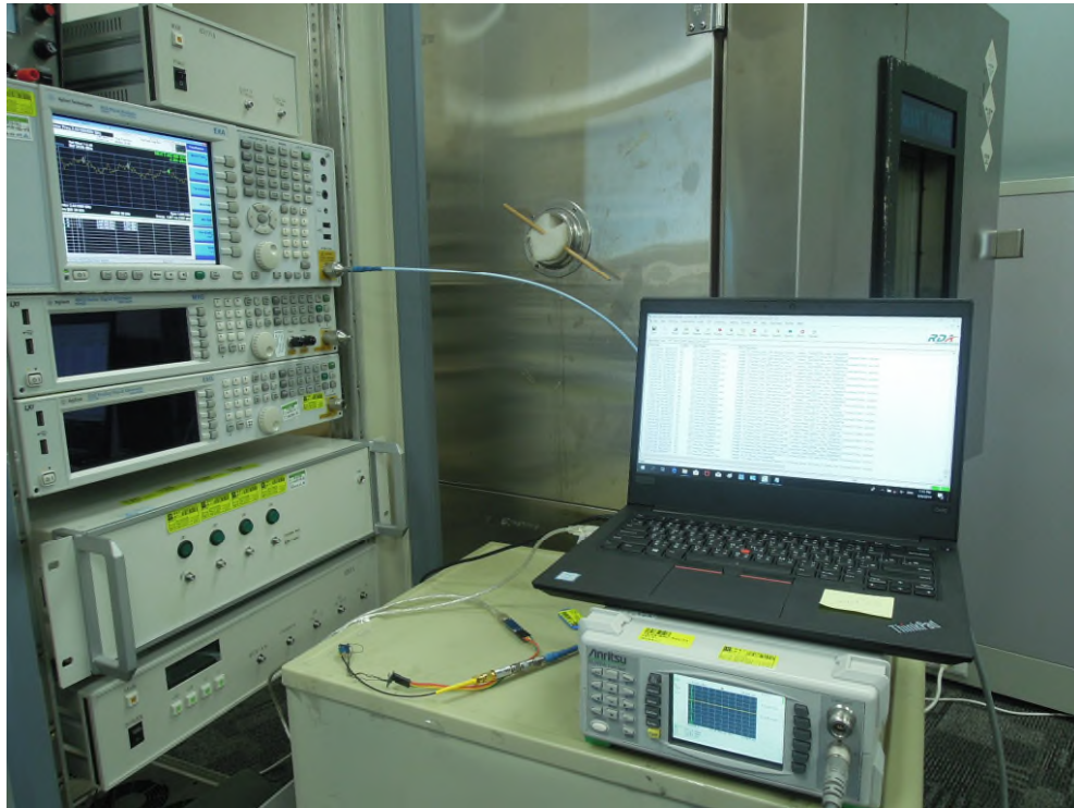
Photograph 5: Set-up for Conducted testing (View 1)
