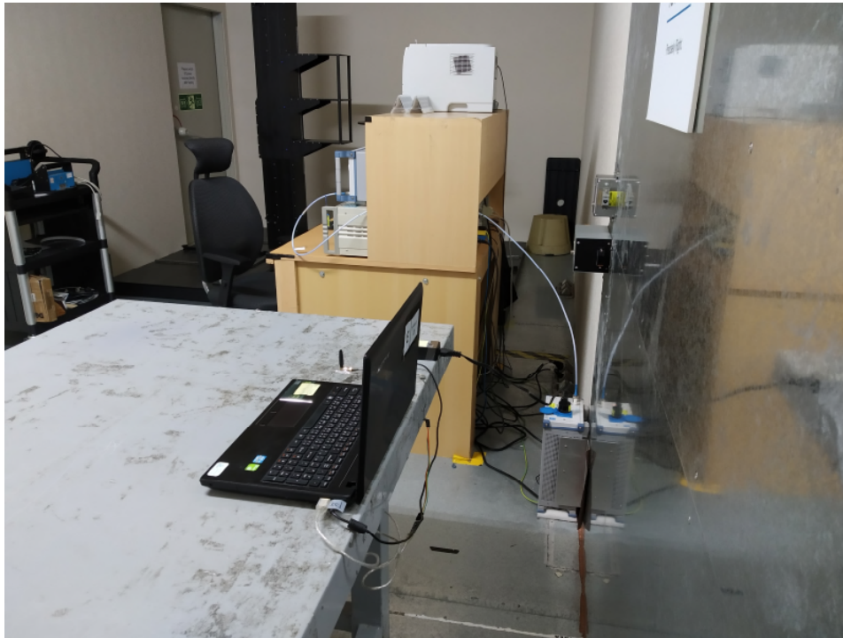
Photograph 7: Set-up for for Mains Conducted testing Back
