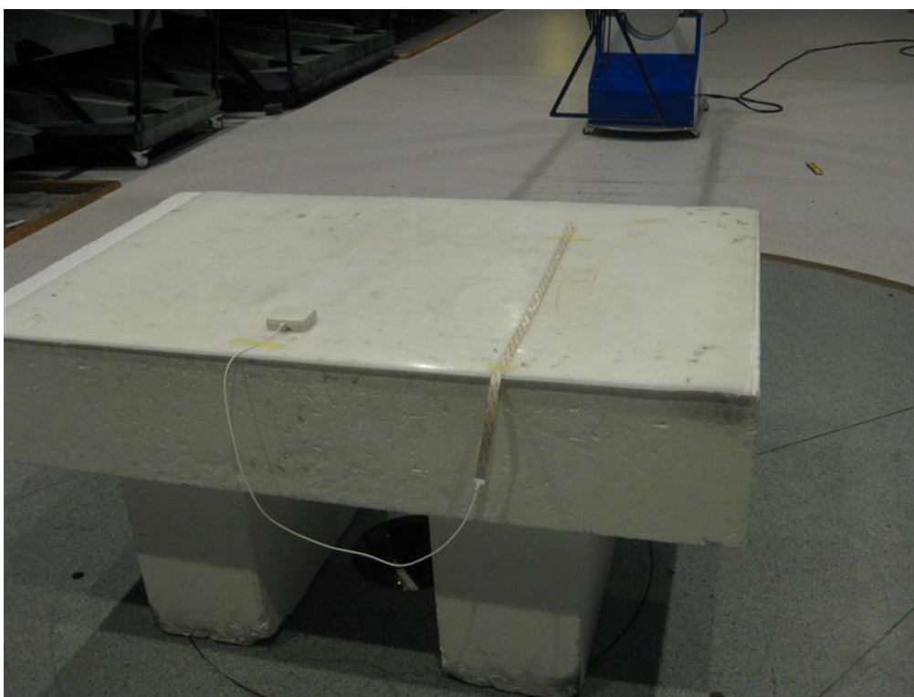
Photo 4.5.2 Test set-up regarding measurement of radiated emission (below 1 GHz).
