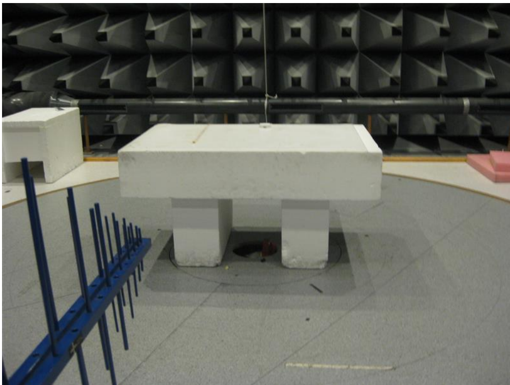
Photo 4.6.1 Test set-up regarding measurement of radiated emission (below 1 GHz).
