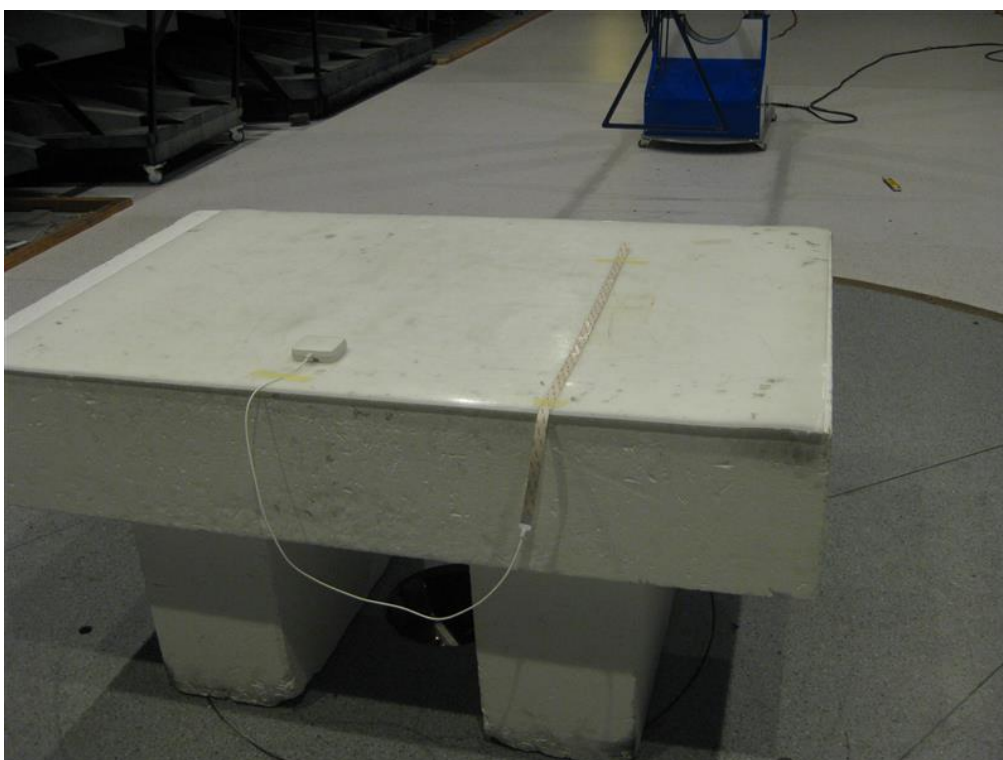
Photo 4.6.2 Test set-up regarding measurement of radiated emission (below 1 GHz).
