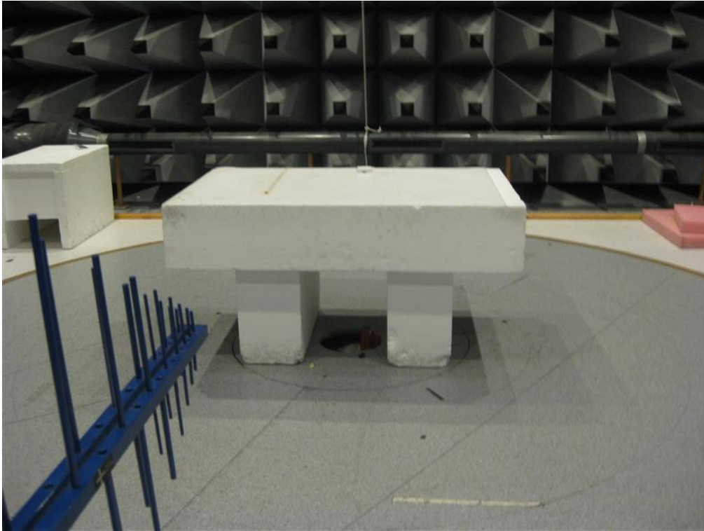
Photo 4.8.1 Test set-up regarding measurement of radiated emission (below 1 GHz).
