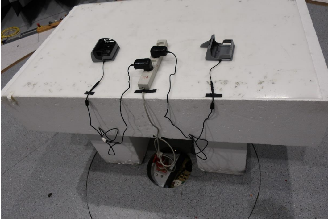
Photo 4.7.2 Test set-up regarding measurement of radiated emission (below 1 GHz).
