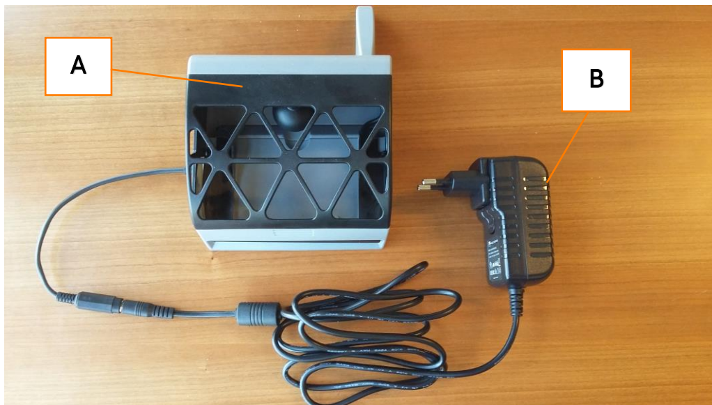
Figure 1: A) Moth configuration seen from the front. B) External power supply.
