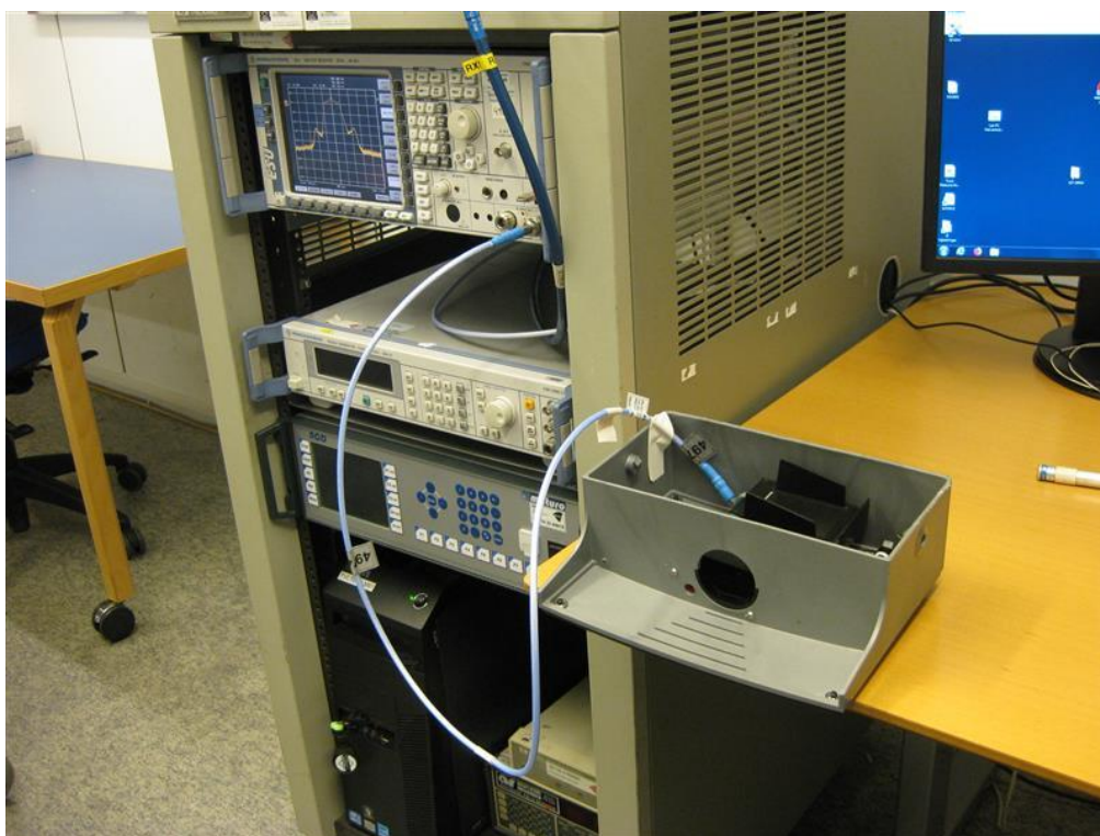
Photo 4.3.1 Test setup regarding measurement of 20 dB bandwidth.
