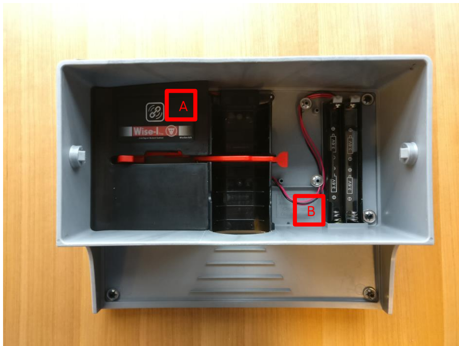
Figure 3: Shows Main enclosure with all the user accessible parts removed. A) is the user interface button, B) is the battery holder.
