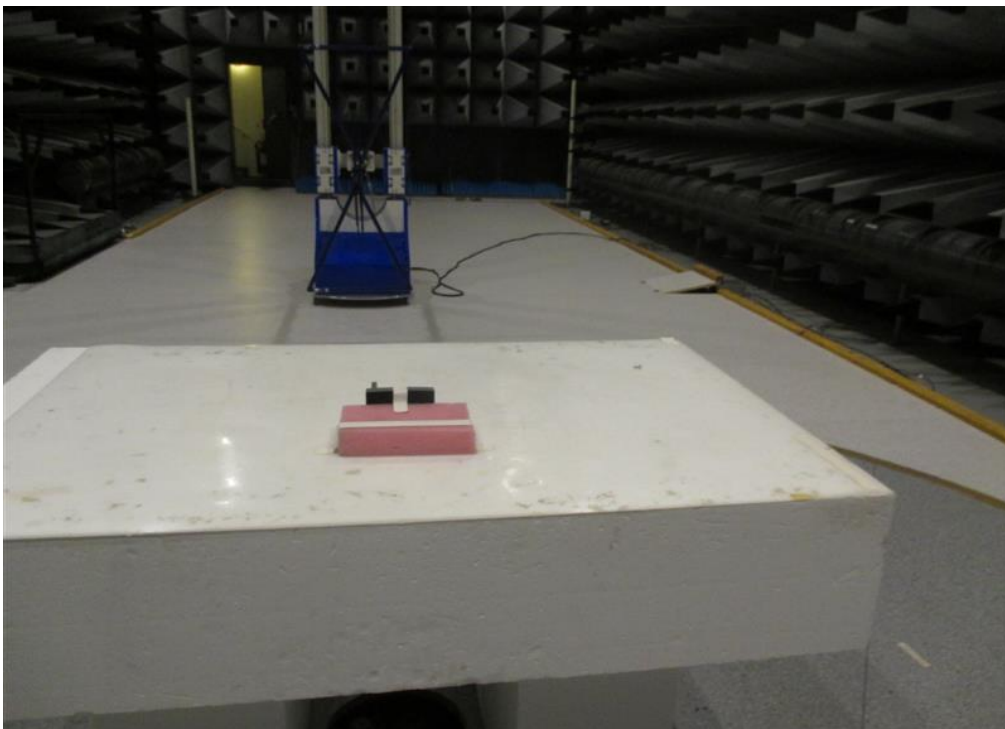
Photo 4.7.2 Test setup regarding measurement of radiated emission (below 1 GHz).
