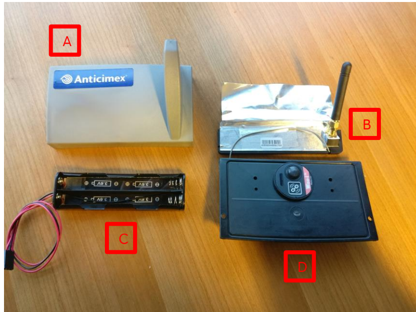
Figure 2: Main components of Smart Eye. A) is the back cover, B) is the antenna holder and PCB enclosure back, C) is the battery holder and D) is the front cover with the PIR sensor.
