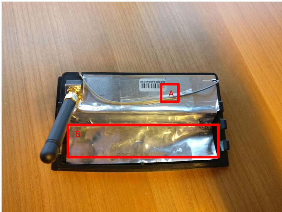
Figure 5: A) Shows the back of Smart Eye with PCB cover mounted. B) cavity for battery holder.
