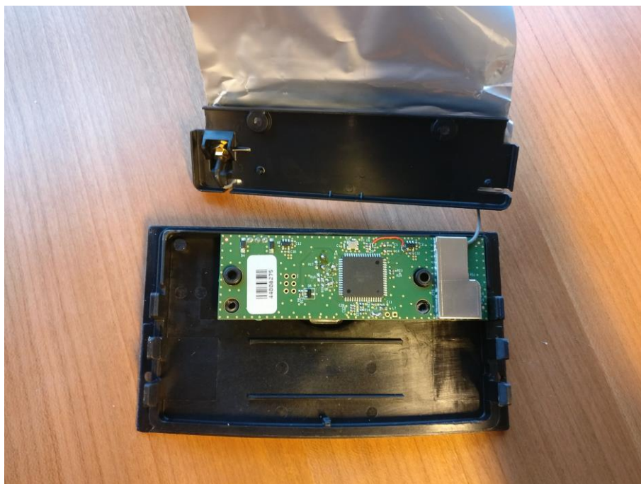
Figure 4: Shows the PCB mounted on the inside of the front cover
