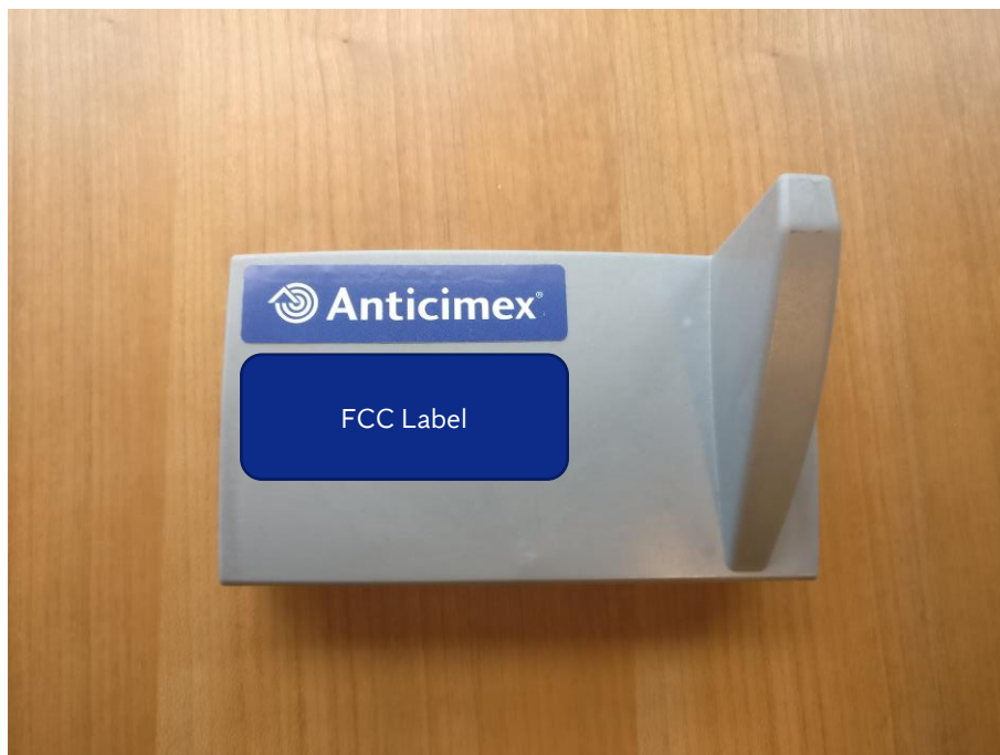
Figure 2: Shows the Smart Eye from the back. The blue rectangle marked "FCC Label" shows the placement of the FCC label
